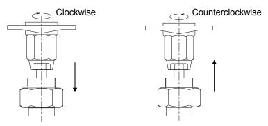
Tighten the adjustment screw to increase pressure
